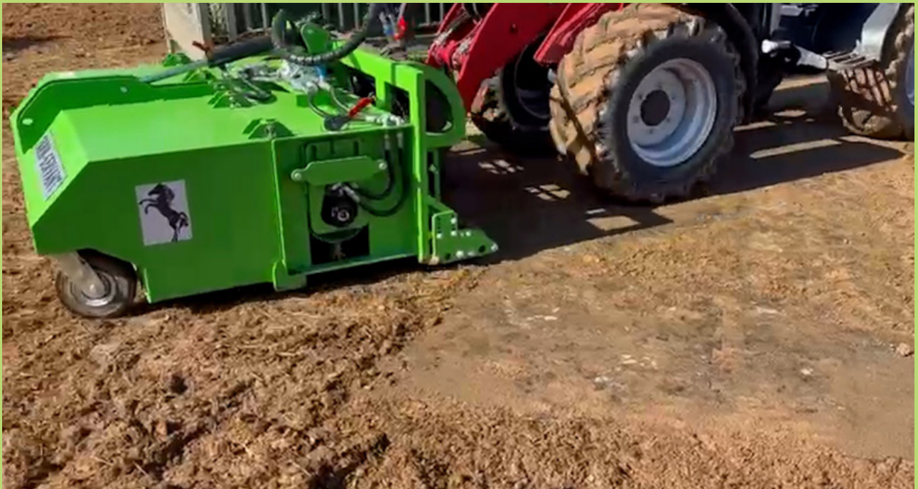
Horse stable „Friesenhof Holler“ in Aurachtal, Germany: Manure removal with the mobile „Farm Servant“ vacuum system in an open stable, around a hay feeder on a stabilized surface laid with BELMONDO paddock mats
